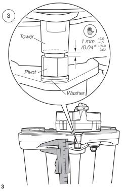
Measure the distance between the top of the tower and the pivot with a slide gauge. This is just a first rough estimation of the distance, see figure.
